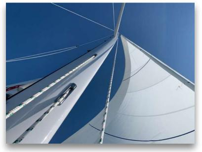
The carbon-fiber mast and the carbon-fiber boom are fabricated by sister company AMP Spars, which builds all the masts for Tartan's complete line-up. The weight savings and stiffness given by carbon-fiber allow for a simple, single spreader, deck stepped fractional rig. The standing rigging is tried and true wire while the running rigging is a sensible mix of yacht braid and higher tech cordage where needed.
